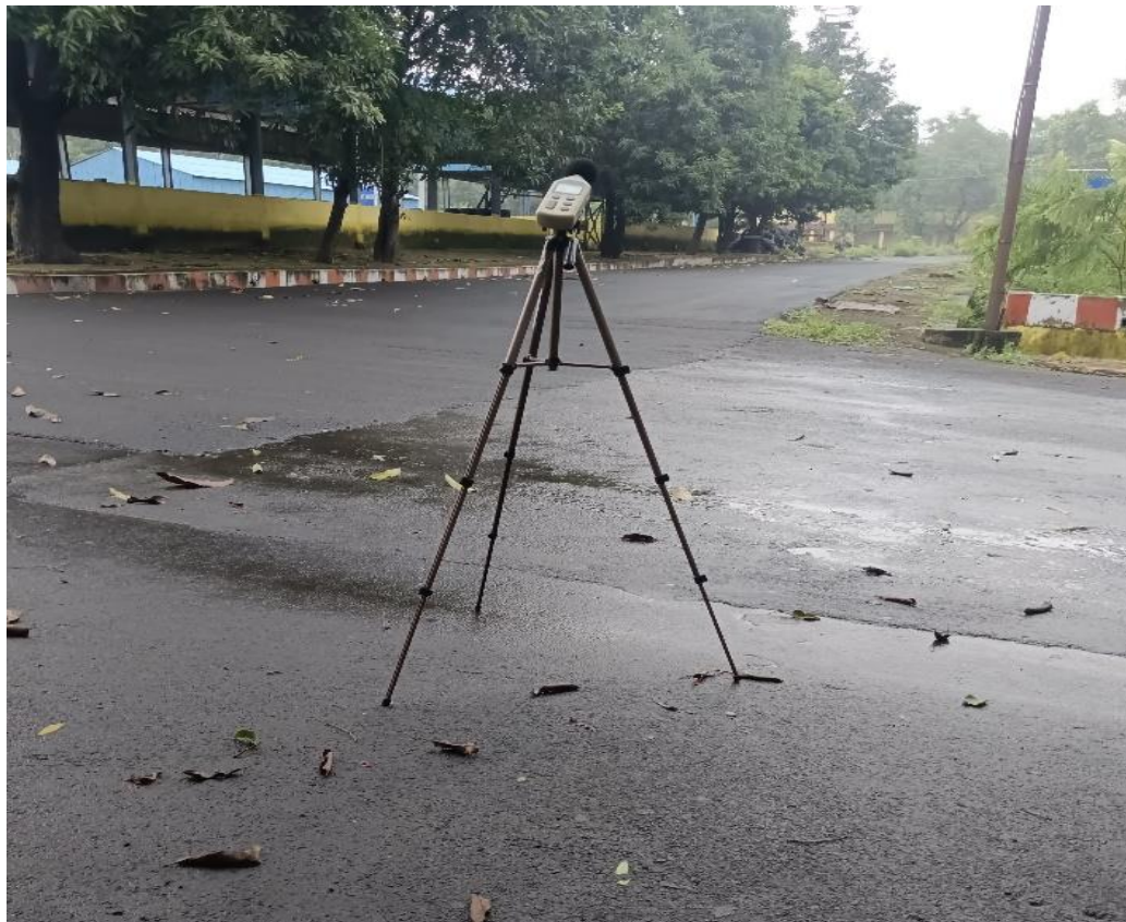
Fig: showing noise measurement at TCF
